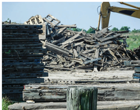
POST JOB CONDITION OF WOOD VERSUS COMPOSITE MATS
